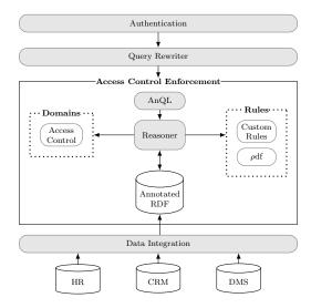
Figure 7.1.: RDF Data Integration and Access Control Enforcement Framework
